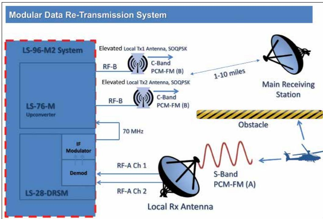
at 70MHz, which can be configured to provide data rates up to 40Mbps from internally derived data patterns.
